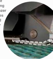
**An optional torsion bar with quick-adjust casters** (shown above) adds rigidity for double- and triple-length forks. Each caster can easily be adjusted to compensate for normal drive tire wear. Simply loosen the lock nut and adjust the caster height with an Allen wrench.
