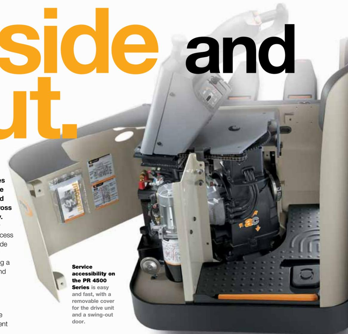
**Service accessibility on the PR 4500 Series** is easy and fast, with a removable cover for the drive unit and a swing-out door.
