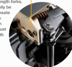
**The lift linkage system** features massive steel construction throughout, including the largest and heaviest tension bar in its class to prevent buckling in the event of a severe impact.
