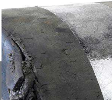
Hysteresis- Evidence of melted material, tread/ poly could have internal bulging across face
