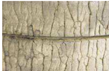
Drive Tires With Fatigue Cracks
