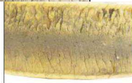
Caster Wheel With Fatigue Cracks
