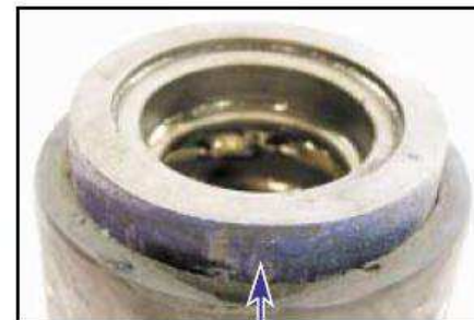
Bond Failure (Hub has been shifted to show hub and tread are completely separated)
