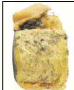
Hysteresis- Evidence of melted material, tread/ poly could have internal bulging across face
