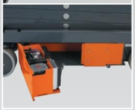
The hydraulic and controller section is easily accessed on a swing out tray, keeping service time to a minimum.
