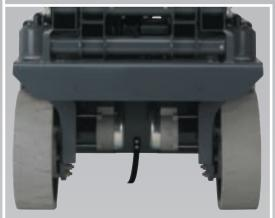
The Aichi AC drive system features AC Brushless motors to create a virtually maintenance free drive system.
