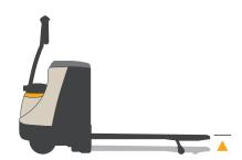
**Lift cutout at full lift** stops the motor once full lift is reached. This reduces energy consumption and extends component life.
