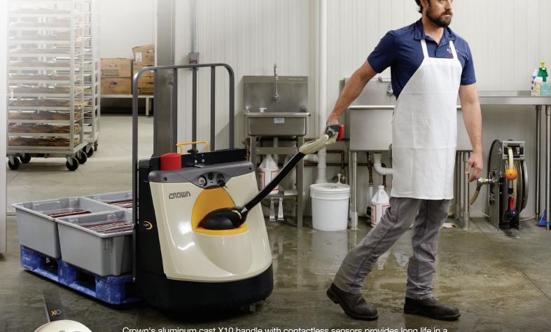
Crown's aluminum cast X10 handle with contactless sensors provides long life in a variety of challenging environments such as wash down, freezer/cooler and meat processing applications. The IP67 Ingress Protection rating ensures the X10 handle is dust-tight and protected against the harmful ingress of water as described in the IP code.
