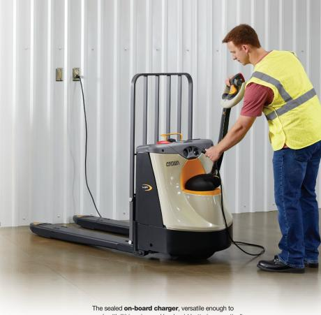
The sealed **on-board charger**, versatile enough to work with lithium-ion and lead-acid batteries, practically eliminates contamination entry which can result in failure.
