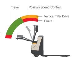
Crown gives operators control to handle the task at hand. When maneuvering a load, the position speed control enables operators to move the handle in near vertical position while engaging traction at creep speed. When operating in tight spaces with the handle completely vertical, the vertical tiller drive function allows for fine-tuned positioning.
