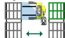
Standing to the side of the stacker eliminates the risk of being trapped or crushed whilst allowing the Combi-WR to operate in very narrow aisles.
